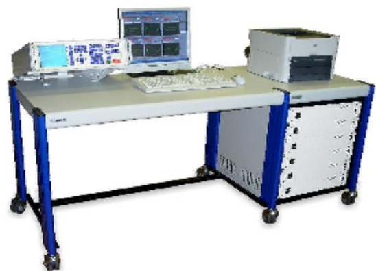
Example of the OT 248 terminal together with a 6-channel PD detector integrated into an operating desk.
