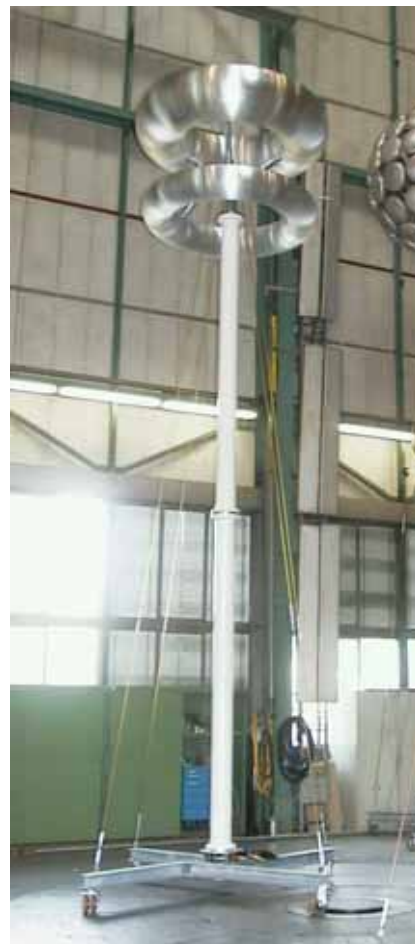
2400 kV impulse voltage divider
