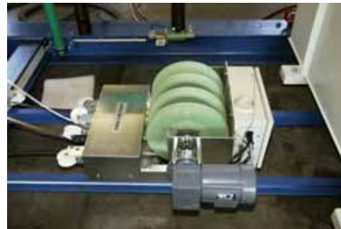
Motorised safety earthing system
