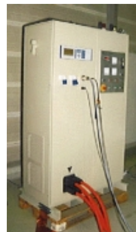
Control unit TKMT for on-site tests.
