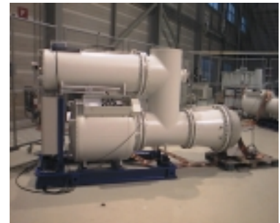
Test system in the works with encapsulated coupling capacitor and connection flange.
