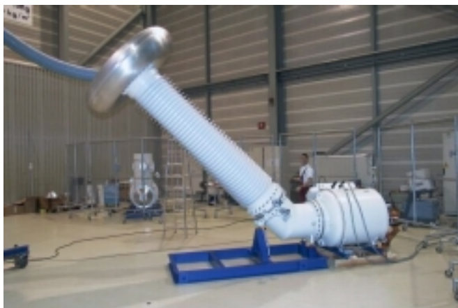
„On-site“ test system with SF6 - air bushing.
