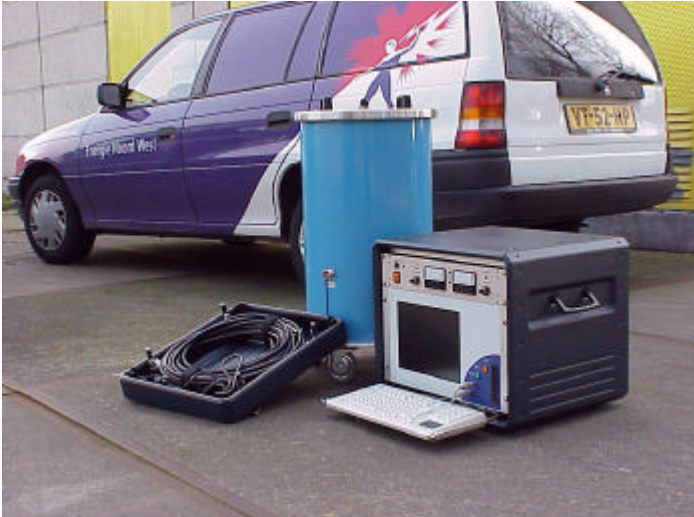
Figure 6 Energie Noord West in Alkmaar, Netherlands have instigated a review of their MV cable network using OWTS ®
