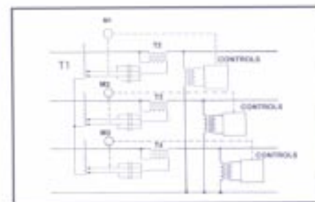
FIG. 6 BUCK/ BOOST, THREE PHASE INDIVIDUAL PHASE CONTROL
