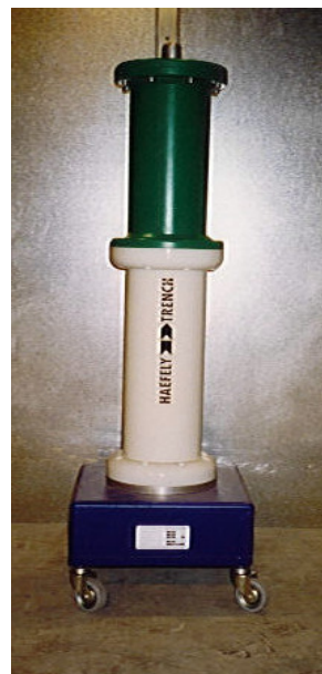
Standard capacitor 100 kV
