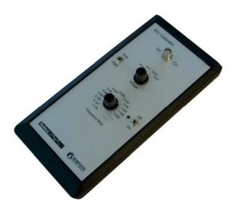
The RIV calibrator is a battery powered hand held instrument needed in the calibration process of the DDX9121 RIV system.
