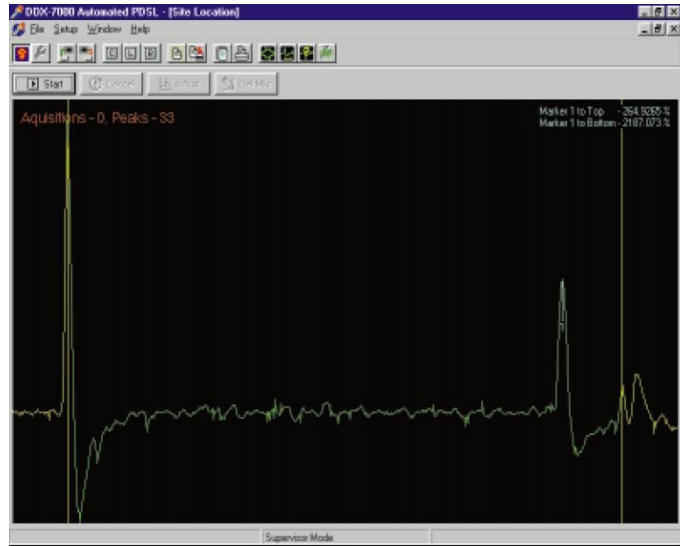
This 2452 ft cable had PD measuring 12pC in magnitude. This fault was easily detectable by adjusting the trigger level in the PDSL software program to locate lower level faults. Note that in doing so, a small amount of background noise is displayed. The Hipotronics PDSL found the fault 265 feet from the top of the cable. The customer cut around the PD site. The cable was retested and passed. Further analysis by the customer indicated that the fault was located at 265.5 feet, an accuracy of much better than .1%.
